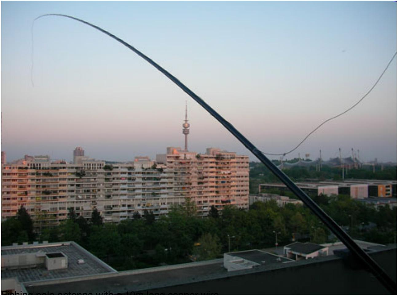
Fishing pole antenna with a 10m long copper wire...
